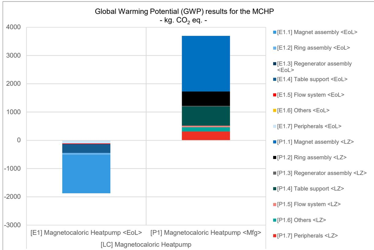
Figure 9 - LCA results for the production (A1-A3 modules) and End-of-Life (modules C+D) of the MCHP
