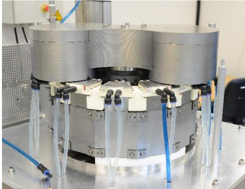
*Figure 4 - The magneto-caloric heat pump*
