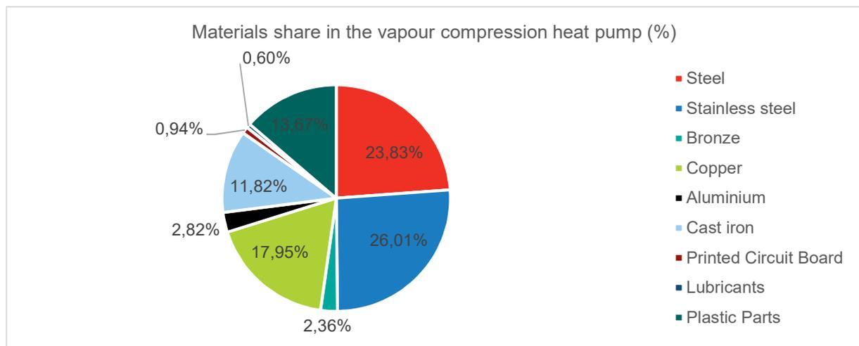
*Figure 6 - Share of materials in the vapour-compression heat pump*
