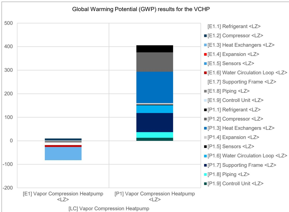
Figure 10 - LCA results for the production (A1-A3 modules) and End-of-Life modules (C+D) of the VCHP. [E] – End-of-Life, depicts the End-of-Life models for each assembly and for the whole technology; [P] – Production, depicts the Production models for each assembly and for the whole technology; [LC] - Life Cycle; <EoL> - End-of-Life
