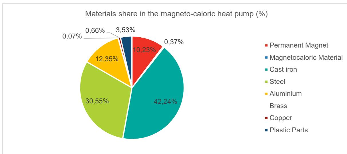
Figure 5 - Share of materials in the magneto-caloric heat pump
