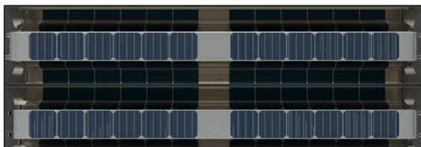
*Figure 2 - Preliminary PV cell string layout*
