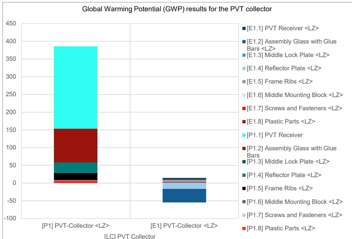
*Figure 8 - LCA results for the production (A1-A3 modules) and End-of-Life (modules C+D) of the PVT collector. [E] – End-of-Life, depicts the End-of-Life models for each assembly and for the whole technology; [P] – Production, depicts the Production models for each assembly and for the whole technology; [LC] - Life Cycle; <EoL> - End-of-Life*
