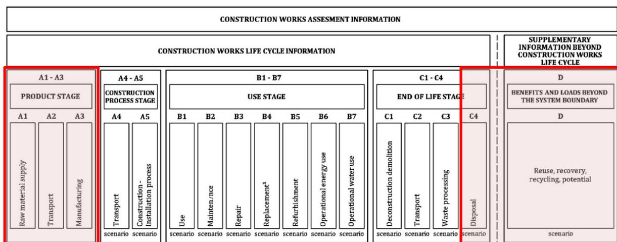
Figure 7 - System boundary for the LCA of the technologies based on EN 15804:2012+A1:2013/FprA2:2019 (E)
